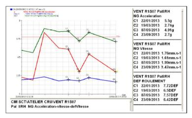
Fig. 12. Curve trend of accelerating loose bearing NG
