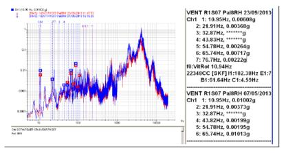
Fig. 13. Spectral analysis of floating bearing
