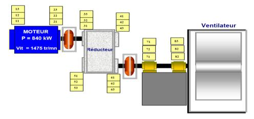
Fig. 5. Block diagram of the fan dispositive
